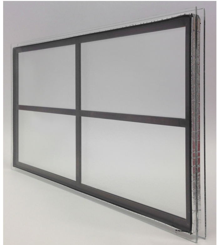
A sample of the leaded glass inserted as the center pane of a triple pane assembly
