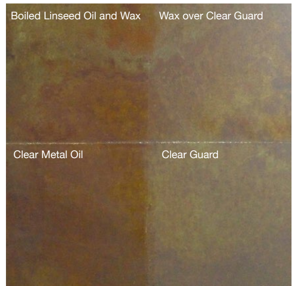
Ferric Nitrate & Japanese Brown. We experimented with a few combinations to achieve desired effects. This sample combines the luminescence of Japanese Brown with the mottled appearance of Ferric Nitrate.
