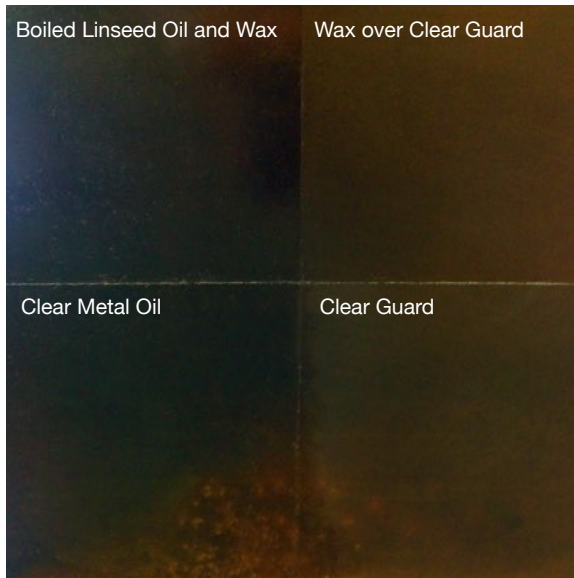
Antiquing. Instant reaction, luminescent golden rust. Easy to gain consistent results. Boiled Linseed Oil and Clear Metal Oil show the most depth in this sample.
